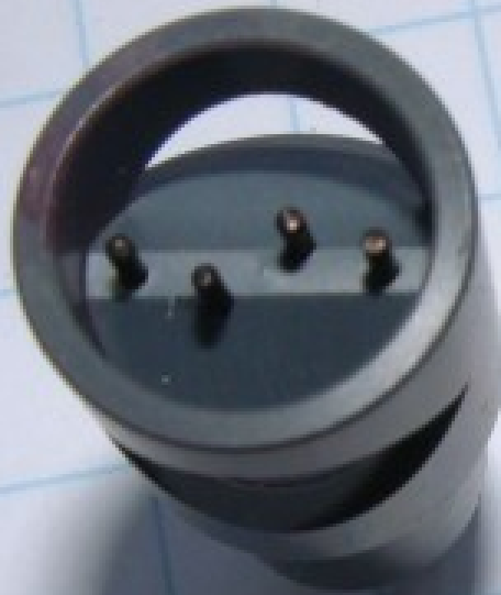
Operational Conductivity Sensor Note black coating
