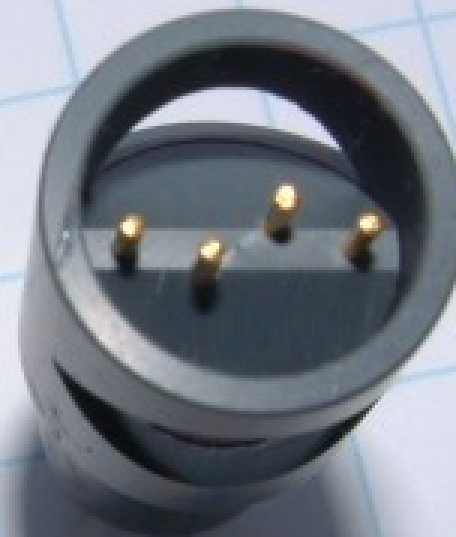
Bare Metal Conductivity Sensor Needs platinizing
